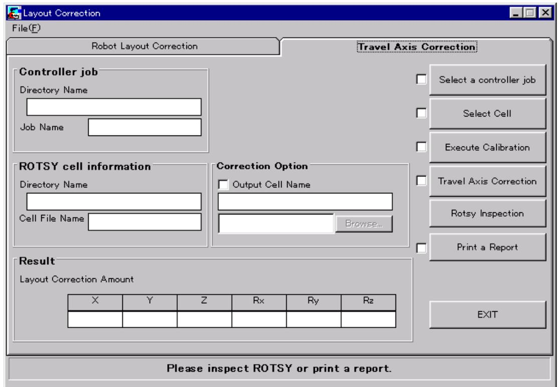
Fig. 2.5.11 "Layout Correction" Screen for Travel Axis Tilt Correction
