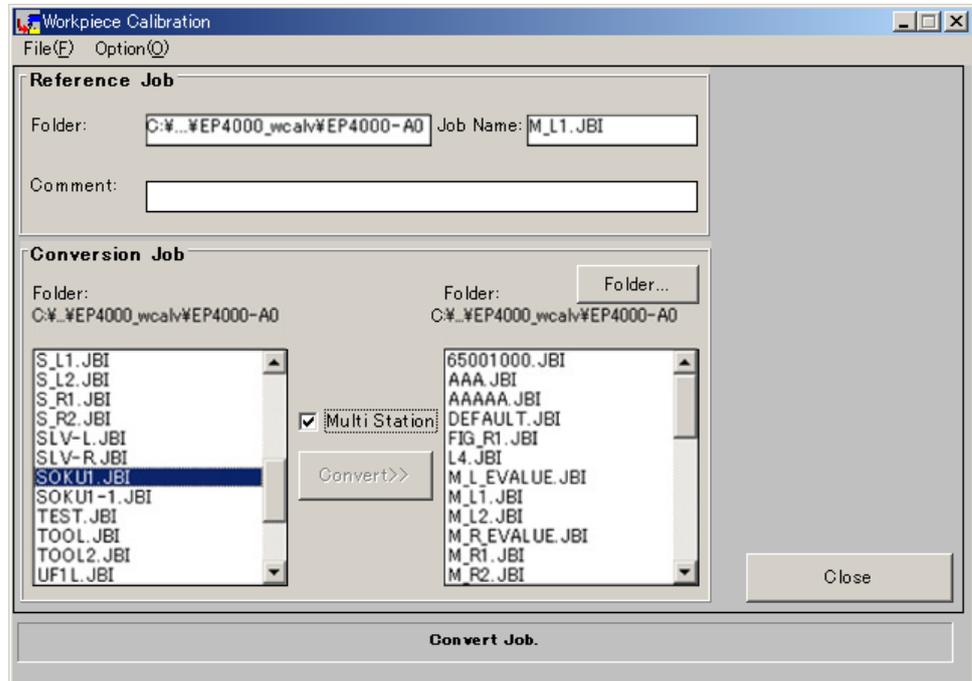
Fig. 2.4.10 “Workpiece Calibration” Screen for Job Conversion
