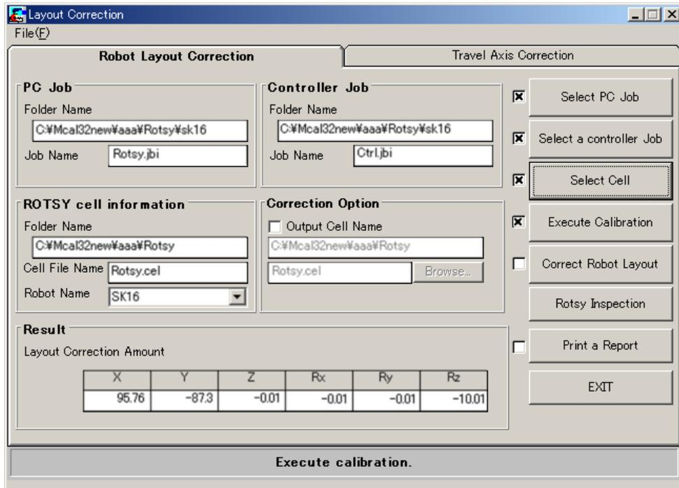
Fig. 2.5.6 "Layout Correction Amount" Screen for Robot Layout Correction
