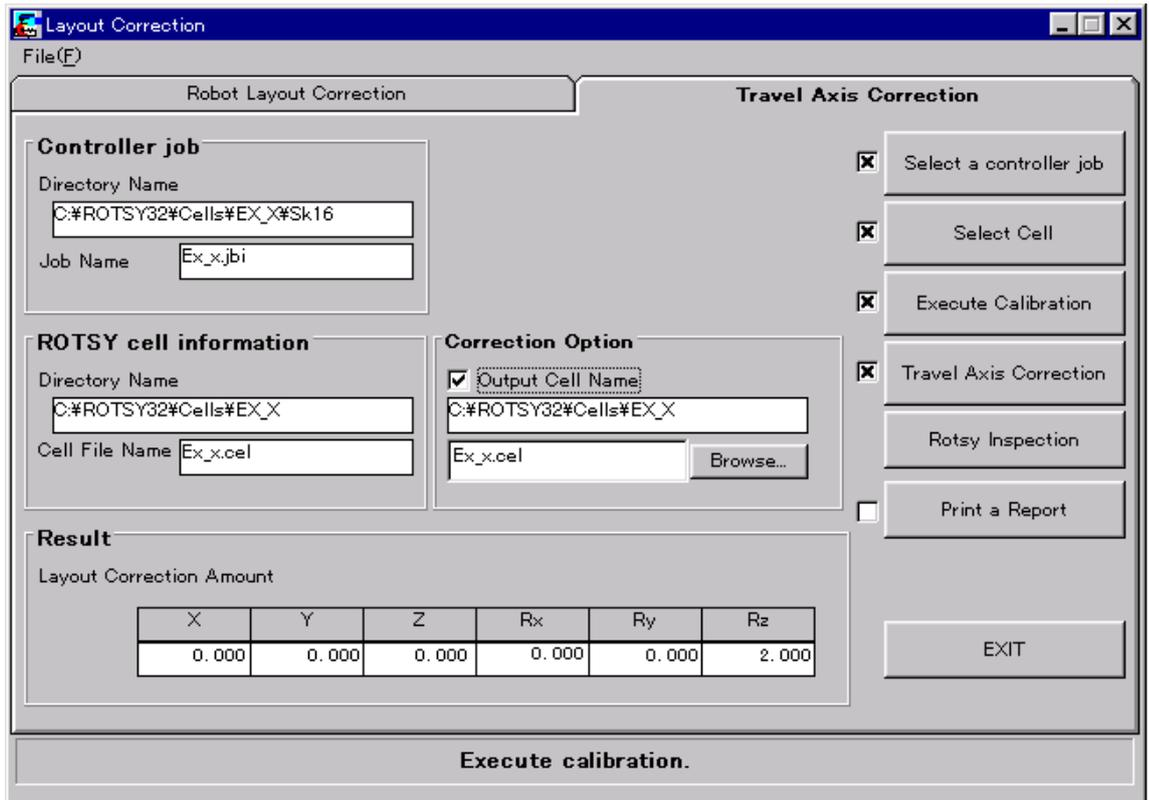
Fig. 2.5.16 "Layout Correction" Screen for Travel Axis Tilt Correction
