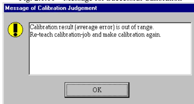
Fig. 2.1.12 Message for Failed Calibration
