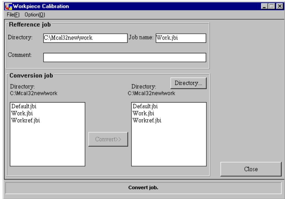
Fig. 2.4.7 "Workpiece Calibration" Screen for Job Conversion
