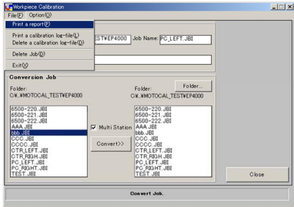
Fig. 2.4.12 “Workpiece Calibration” Screen for Job Conversion When Selecting form the File Menu
