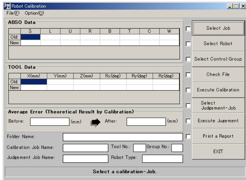
Fig. 2.1.5 "Robot Calibration" Screen
