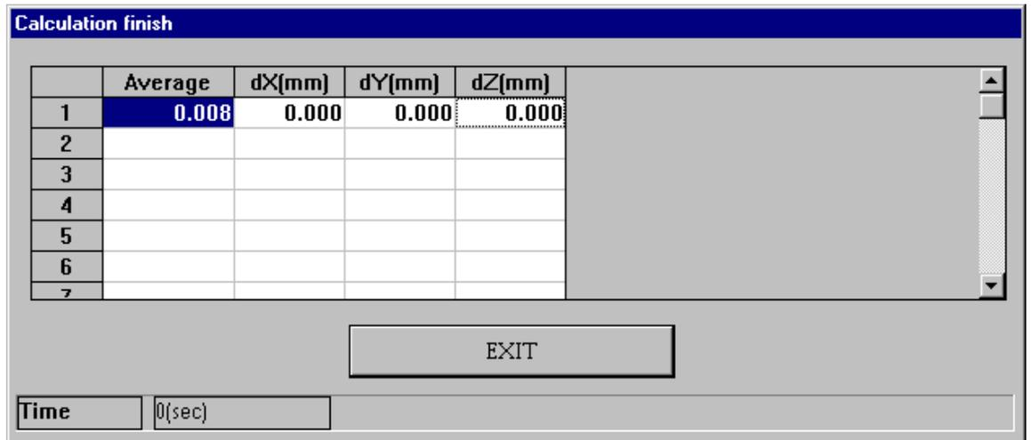
Fig. 2.2.6 "Calculation finish" Screen for Tool Calibration Calculation Process
