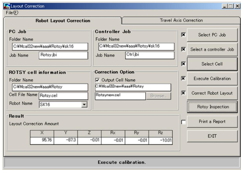
Fig. 2.5.7 "Layout Correction" Screen for Robot Layout Correction
