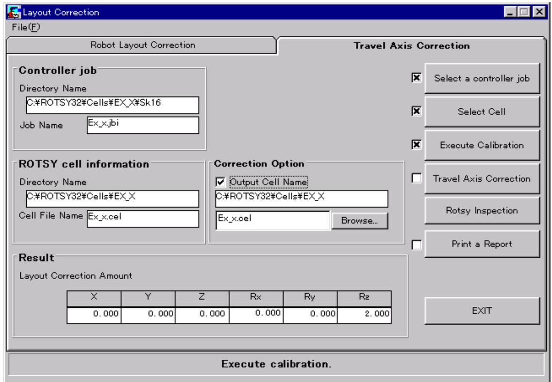
Fig. 2.5.15 "Layout Correction" Screen for Travel Axis Tilt Correction Amounts
