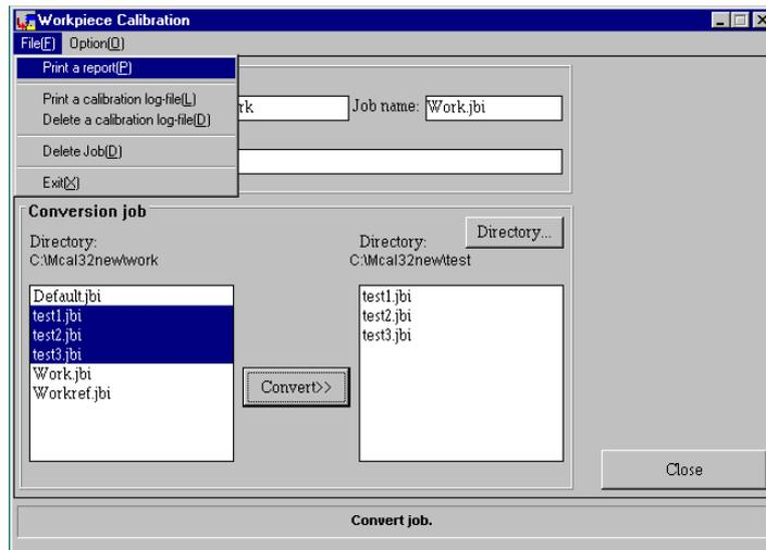
Fig. 2.4.9 "Workpiece Calibration" Screen after Job Conversion (at Selecting from File Menu)
